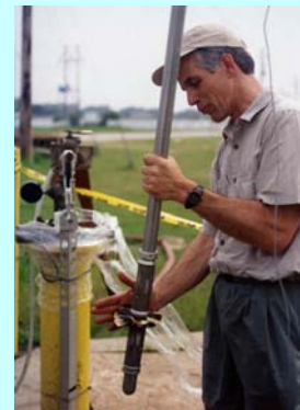
Borehole flowmeter logging by WGNHS to identify possible preferential flow zones
