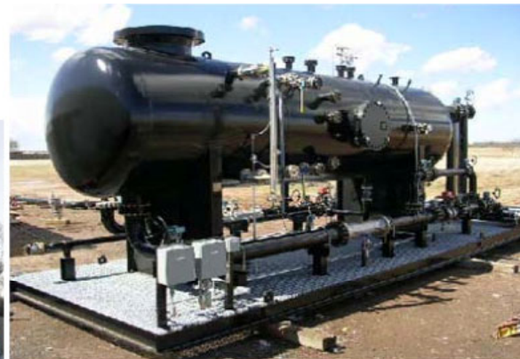
Separator for separating produced fluids (oil, water, and gas)
