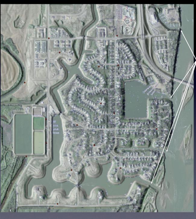
Dikes were built across the mouths of the bays and then pumped to control the water levels within the development.
