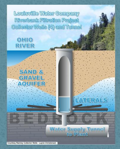
**4** Collector Wells Each shaft ~ 100 feet deep 13 - foot ID8 - 12'' laterals  $Q \sim 15$  MGD each
