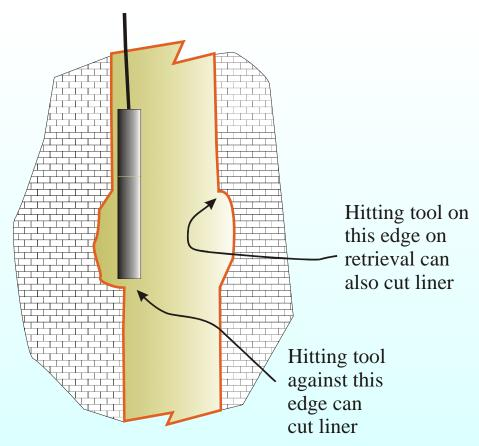
Pad the top and bottom of tools to reduce impact on ledges and damage to liner
