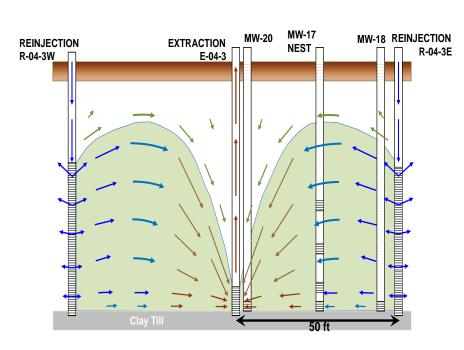
Cell 4 cross section operation flow rates:  $E \sim 0.25 - 3$  gpm per well  $R \sim 0.5 - 1.3$  gpm per well
