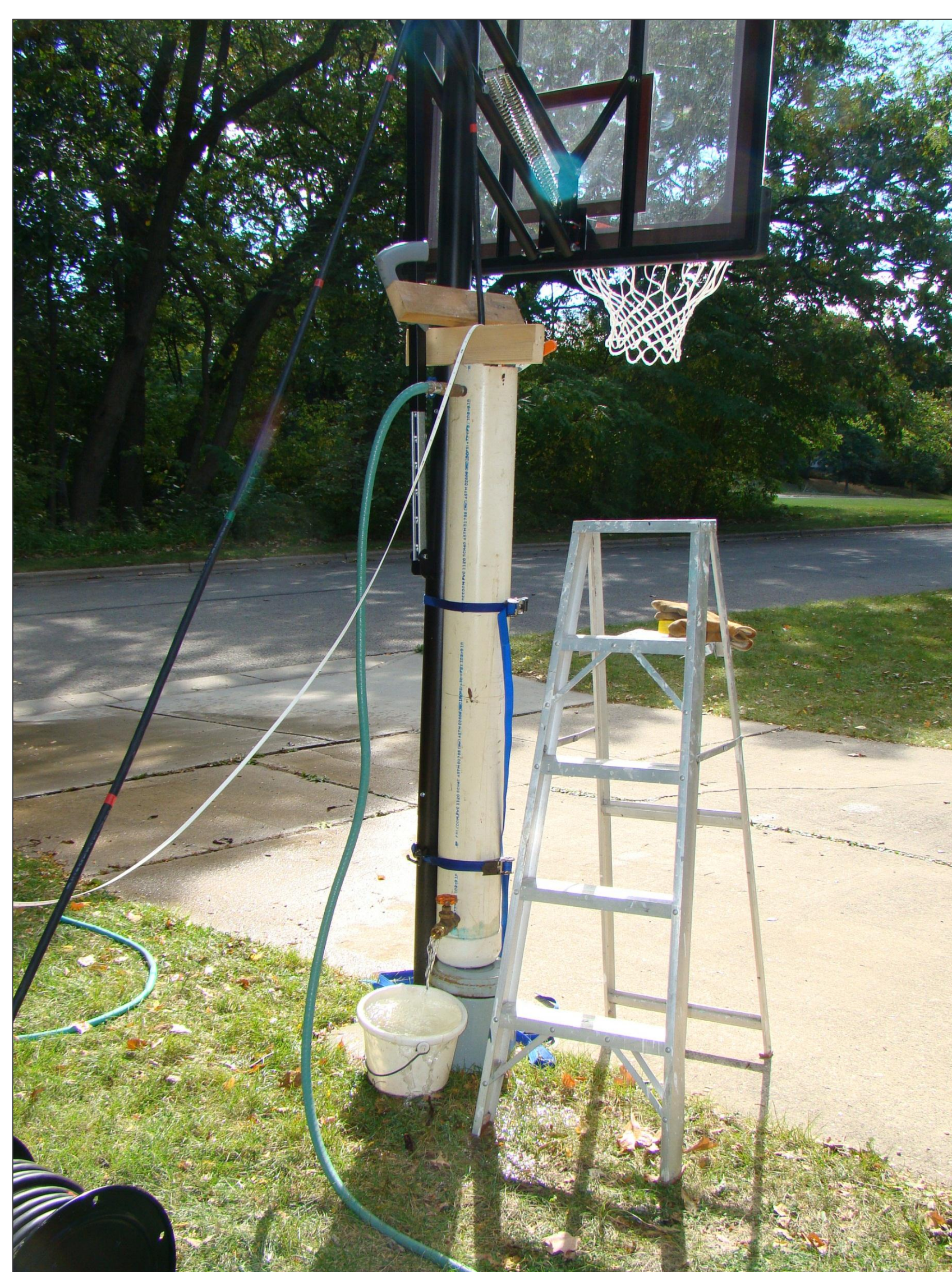
Figure 2e – Experimental well setup with downward flow configuration.
