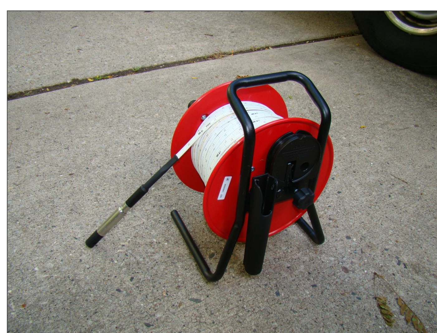
Figure 2c – Water level electric tape with temperature and fluid conductivity probe.
