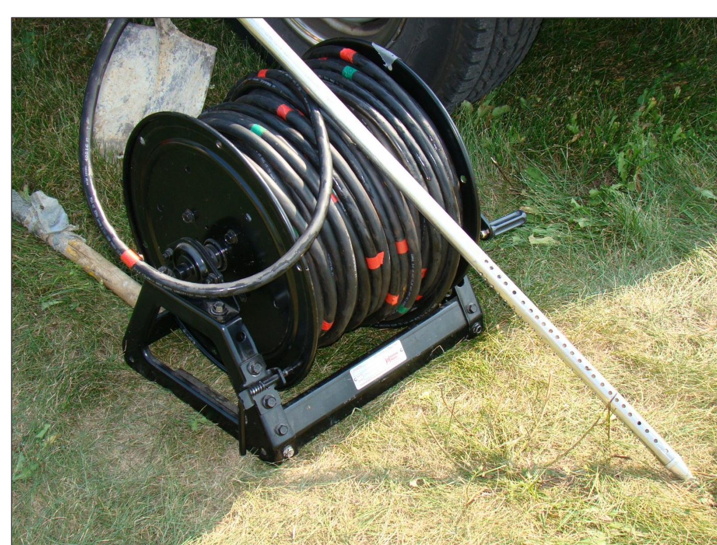
Figure 2a – Photo of heater showing shroud and electrical cord on a spool.
