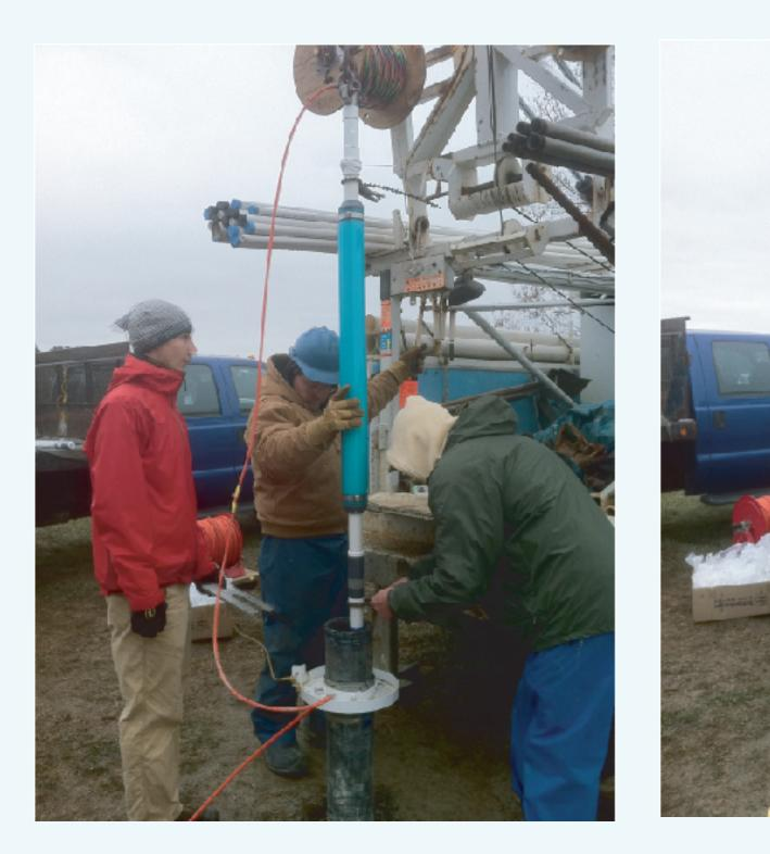
Photographs taken during installation of MLS, showing one of the packers and one of the monitoring
