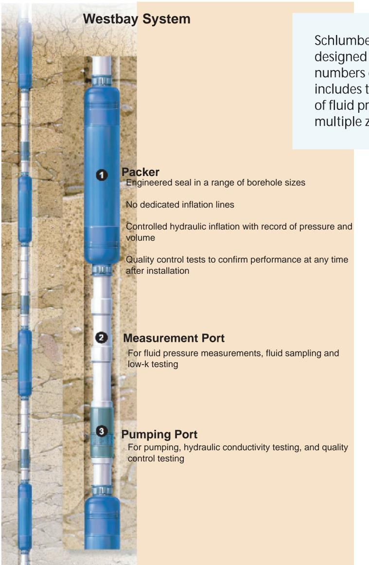
Schlumberger Water Services/ Westbay System is designed for collecting subsurface data at large numbers of discrete positions within a single well. This includes testing of hydraulic conductivity, monitoring of fluid pressure and collection of fluid samples from multiple zones.
