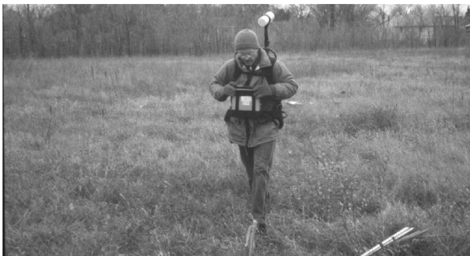
Todd Petersen, Minnesota Department of Natural Resources, Waters Division, conducting a magnetometer survey in November 1998 to search for the buried railroad well, Maplewood, Minnesota
