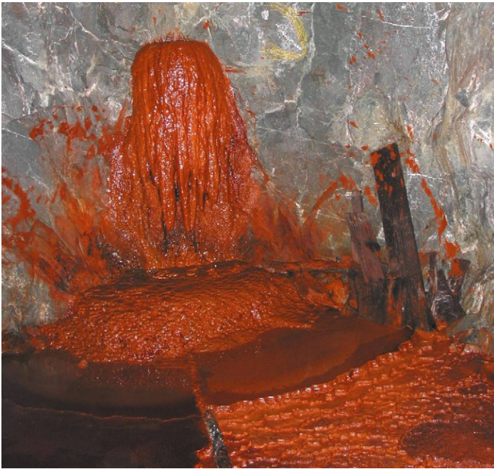
Figure 6. Ferrihydrite drapery and rimstone dams at DDH 962, 27th East Drift.
