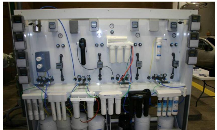
Figure 1: Field test station setup to allow side-by-side evaluation of point-of-use devices.
