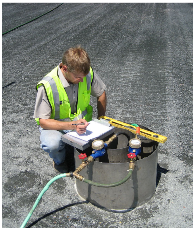
Figure 5. Left: The double-ring infiltrometer being run in a coarse granular base course. Right: Mechanics of the double ring infiltrometer test illustrated in plan view (top) and section view (bottom)
