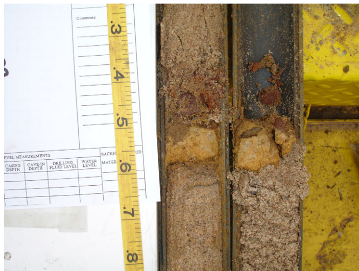
Figure 2. The effect a thin layer of restrictive soil can have on infiltration – in this open split spoon, note the mottled soils above the thin clay layer and the coarse dry sand below.
