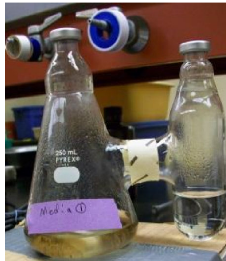
Figure 3: Batch tests were used to determine biodegradation kinetics. (Photo: LeFevre)
