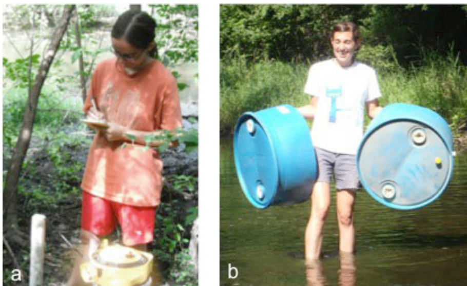
Figure 5. (a) Measuring temperature, level, and conductivity in a shallow well near Minnehaha Creek. (b) Preparing to install seepage meters in Minnehaha Creek.
