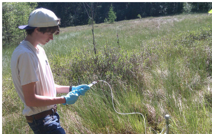
Ryan Streitz extracting water samples from a wetland well in Bemidji.
