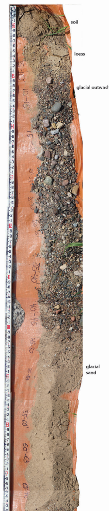
Borehole cuttings from dual-rotary reverse circulation drilling at South Washington Watershed District retention basin
