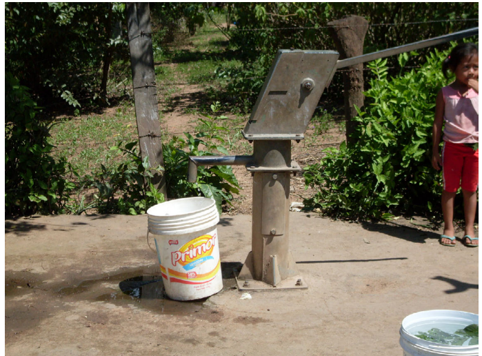
Photo 4. Well with hand pump
