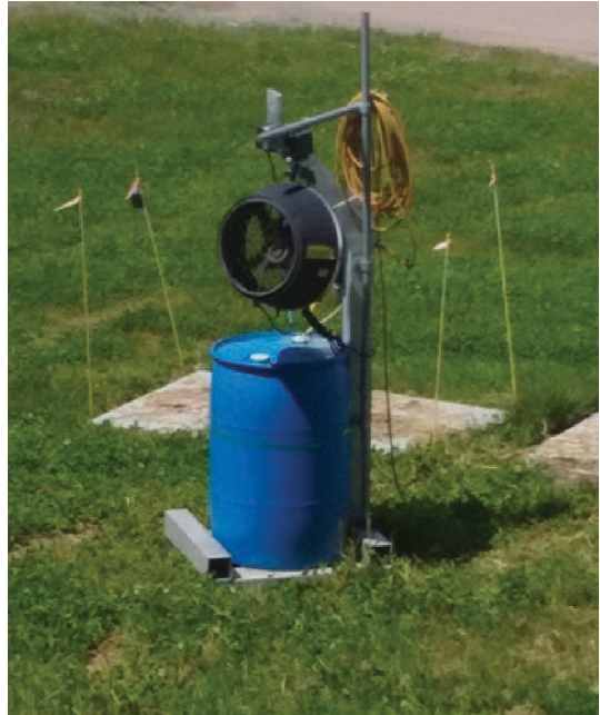
Figure 1. Here is an Odor Fan that sprays a scented mist, this is used as part of the air monitoring to limit the site's exposure on the public.
