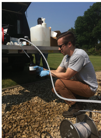
Figure 2. Matthias Wolf fills a 1 liter amber glass bottle from a monitoring well using a submersible pump for the pesticide sampling done in collaboration with MDA.
