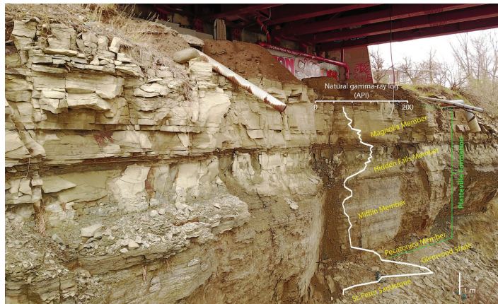
Figure 3. An example natural gamma radiation log and how it correlates to the various strata exposed along an outcrop of the Ordovician-aged St. Peter Sandstone, Glenwood Shale, and Platteville Formation in the Twin Cities metropolitan area.
